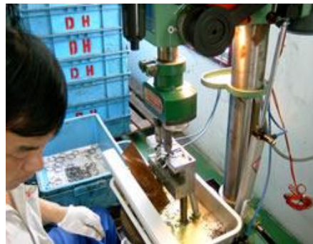
tapping process for stamped part in progress
