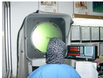
using profile projector for inspection
